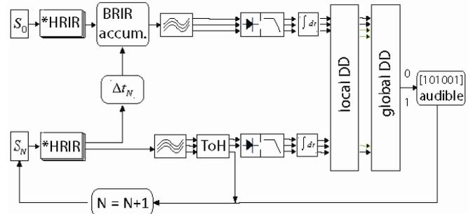
**Figure 1:** Block diagram of the iterative auditory process model of reflection masking in RIRs ( $S_0$  = direct sound,  $S_N$  = current test reflection), see text for further explanation
